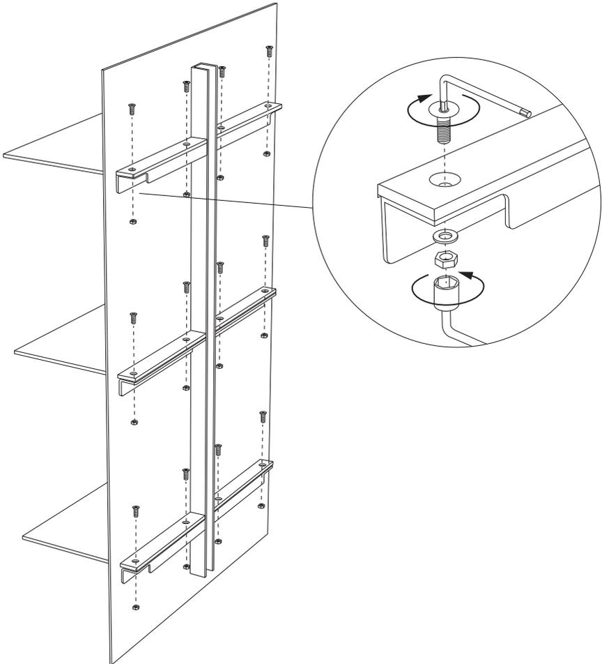
Insert 4 screws (A), 4 washer and 4 bolts on the back of each shelf.
