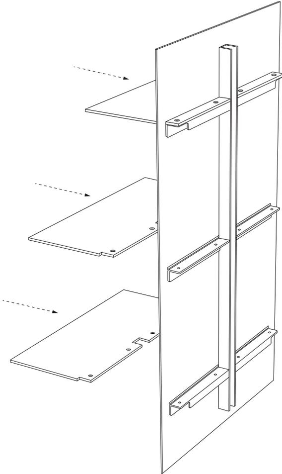
Insert the three shelves into the backplate through the three cut-outs.
