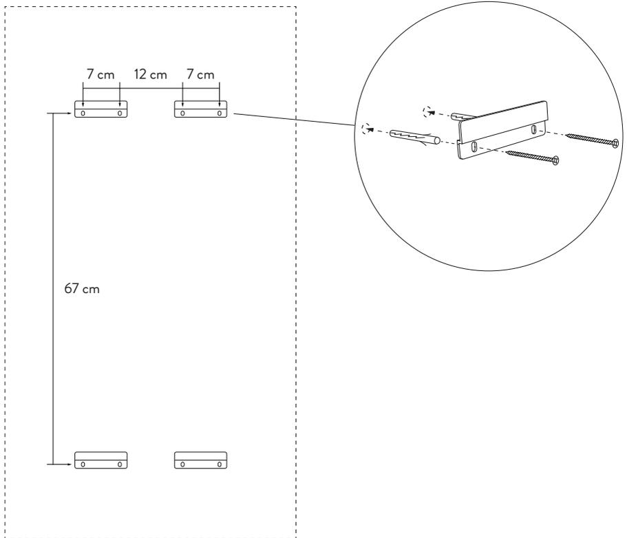
Measure and drill holes for the four wall brackets. Follow the measuring instructions and mount each bracket with two screws (B) and wall plugs.
